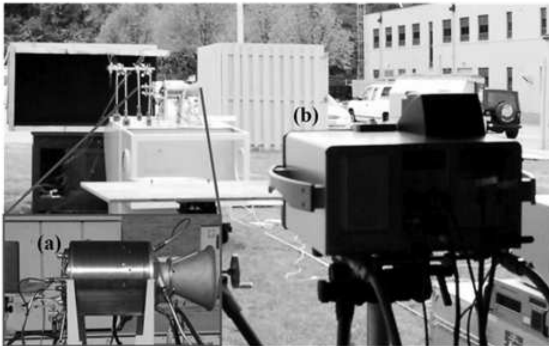
Figure 15. Experimental setup for collecting exhaust data from a turbojet engine (a) with the Telops FIRST-MWE (b). The turbojet engine was filled with diesel fuel and run at a fuel flow rate of 300 \frac{cm^3}{min} .
